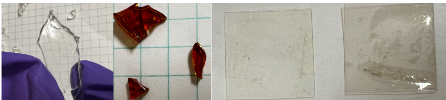
Figure 3.7: Translucency in Durazane1800-DCPO thick films and coatings.
