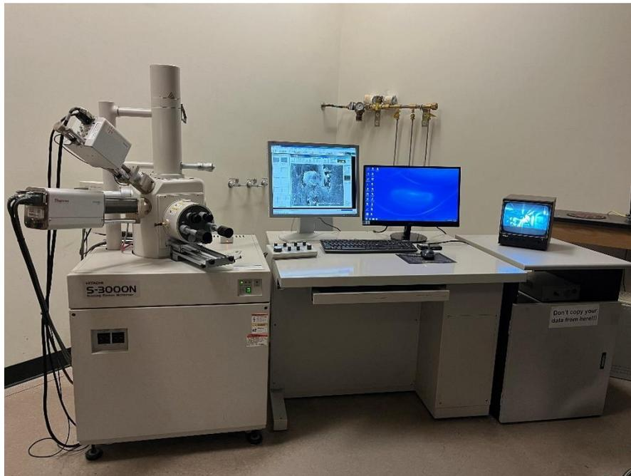
Figure 3-21. SEM/EDS Hitachi model S-3000N.
