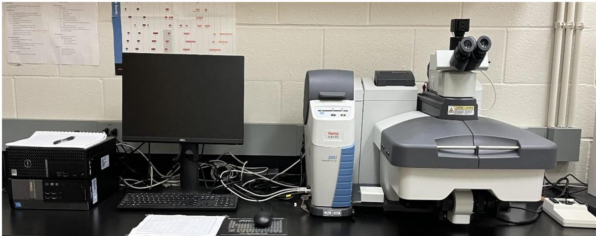
*Figure 3-15. Thermo Fisher DXR3 Raman Spectroscopy*
