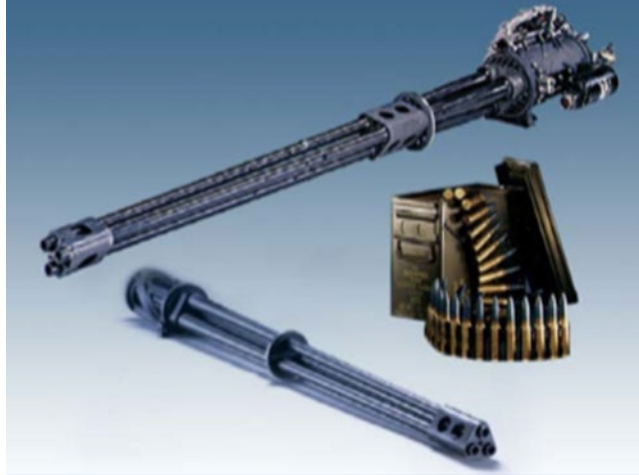
Figure 3.7: XM301 20mm lightweight Gatling gun with ammo
