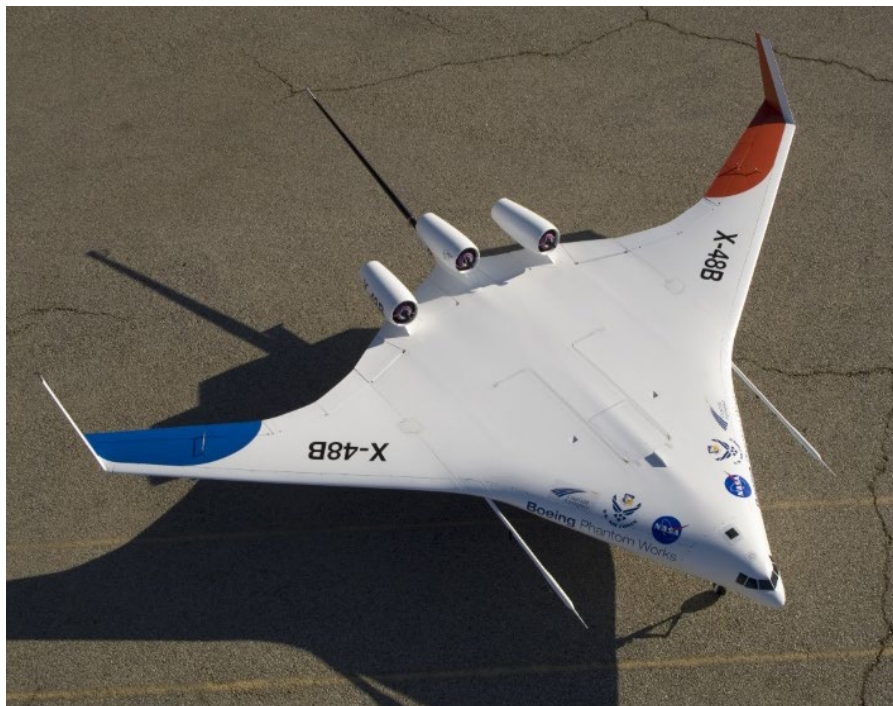
Figure A.4: Blended Wing-Body Configuration Example [12]
