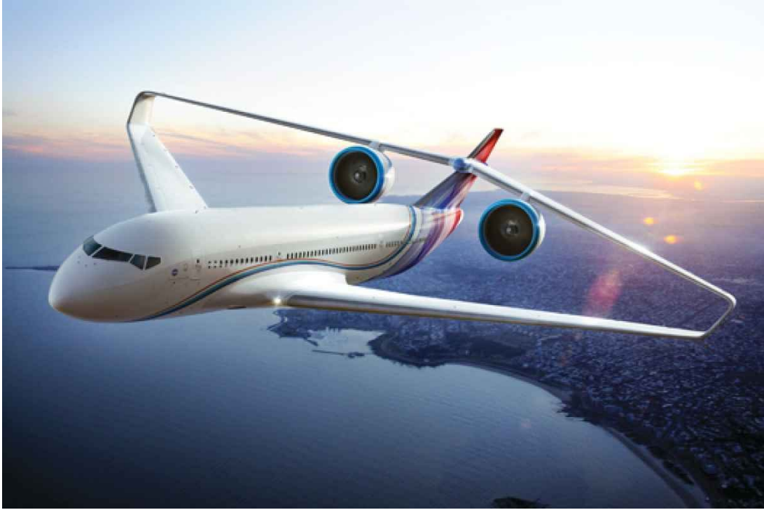
Figure A.3: Joined-Wing Configuration Example [11]
