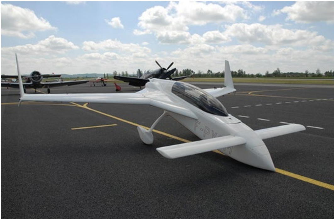
Figure A.2: Canard Configuration Example [10]
