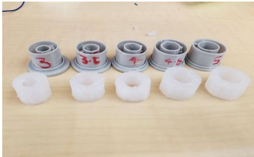
Figure 3.1: Silicone rubber rings of different diameters fabricated with the help of ABS plastic molds
