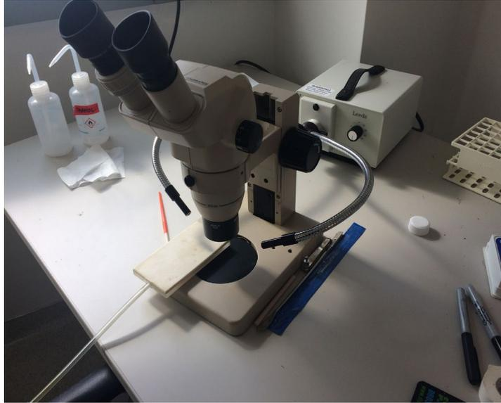
Figure 2.4: Microscope and Carbon Dioxide Pad (White Pad with Tube Attached to the Base of the Microscope)
