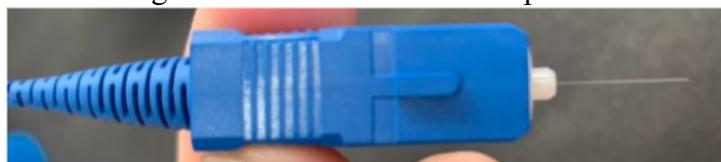
Figure 3.11: Fiber extending through connector
