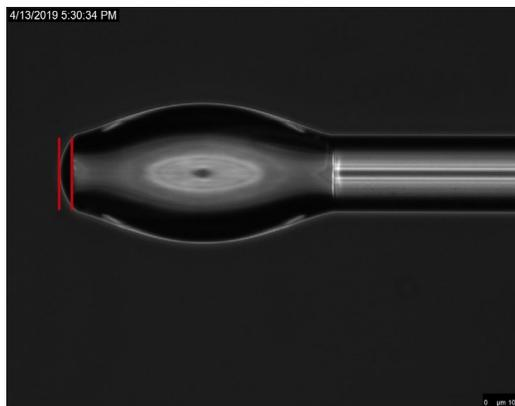
Figure 3.16: Magnified image of the PDMS after curing for 24 hours and gap formed
