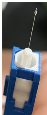
Figure 3.17: Fiber tip coated with epoxy
