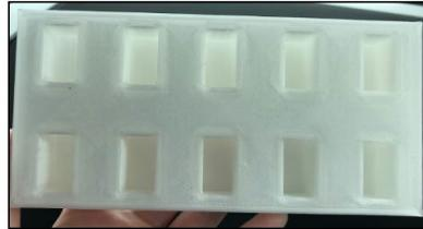
Figure 3.12: Coating tray with top view of various housing units
