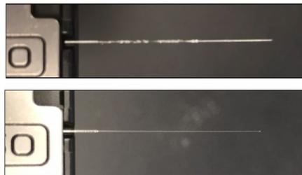
Figure 3.7: Stripped fiber before (top) and after (bottom) cleaning
