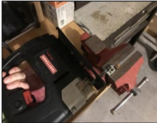
Figure 3.4: Alteration process of SC mating sleeve with jigsaw
