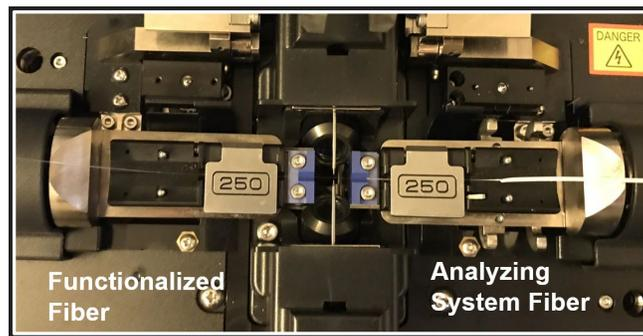
Figure 3.18: Splicing process joining functionalized fiber and analyzing system fiber
