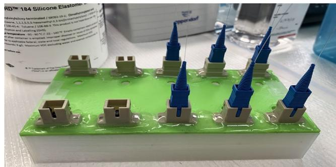
Figure 3.13: Coating tray with mating sleeves and connectors inserted
