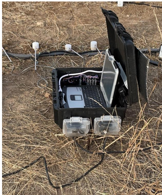
Figure 9: A Data Acquisition (DAQ) Unit placed at the testbed during an experiment. The Toughbook computer, the data flow connections of 5 pin IP68 aviation connectors can also be seen.
