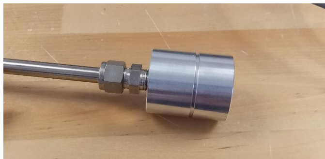
Figure 8: The Stainless-steel holder and 1/4 tubing assembly for INIR-data wire protection
