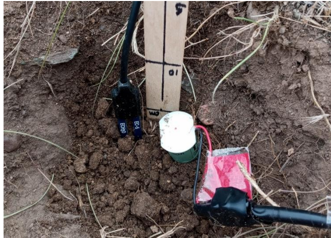
Figure 12: Oxygen sensor installment during a proof-of-concept experiment. The sensor was placed to facing the sensing side downwards. Collocated EC5 soil moisture sensor can also be seen.
