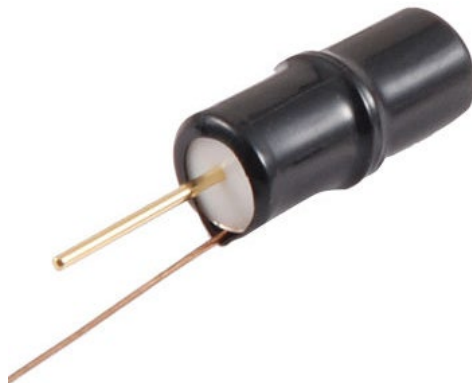
Figure 3.5: A Tilt Switch
