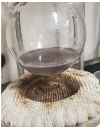
Figure 2.1: PEG-Functionalized CuCy Solution. Prepared solution that should be taken off heat at this point to follow a washing and drying process PEG-Functionalized CuCy
