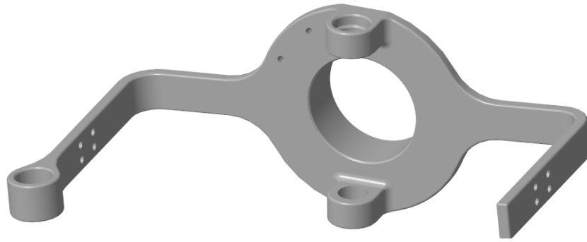
Figure 5.8: Original Steering Knuckle Design
