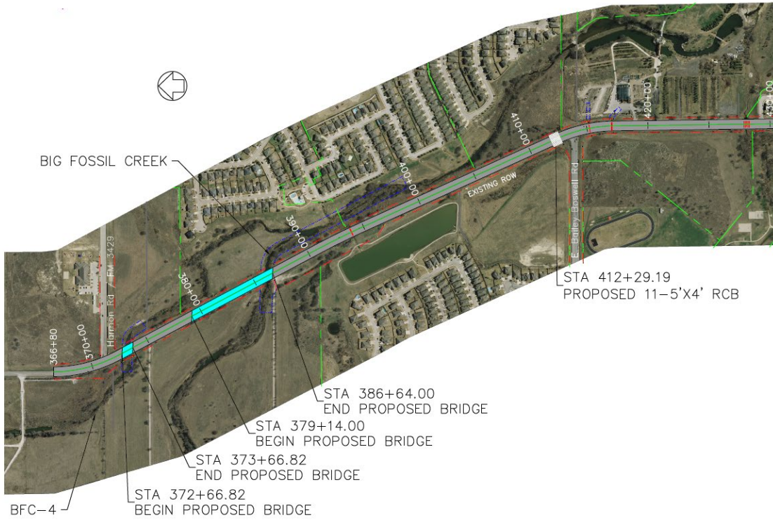
Figure A.2: Layout of Proposed Cross Drainage Structures (Not to Scale)
