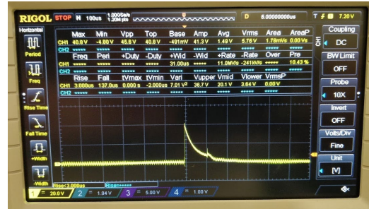
Figure 5.3: 100us Long Output Pulse
