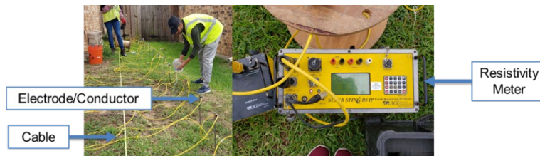
Figure 3.1: ERT Components and Set-Up. Note: VegaMartinez, R. (n.d.). [Photo of Electrical Resistivity Tomography equipment and layout].
