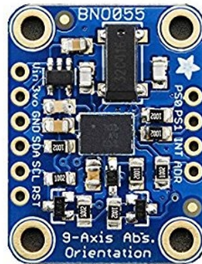
Figure 4.2: Fusion Breakout BNO055 IMU [6]
