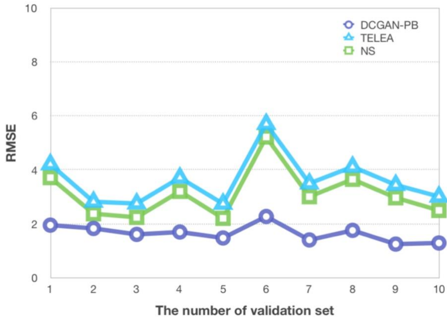
Figure 3.9 RMSE for 10 cross-validation sets by TELEA, NS, and DCGAN-PB methods for (a) high solar activity years and (b) low solar activity years [Pan et al., 2020].
