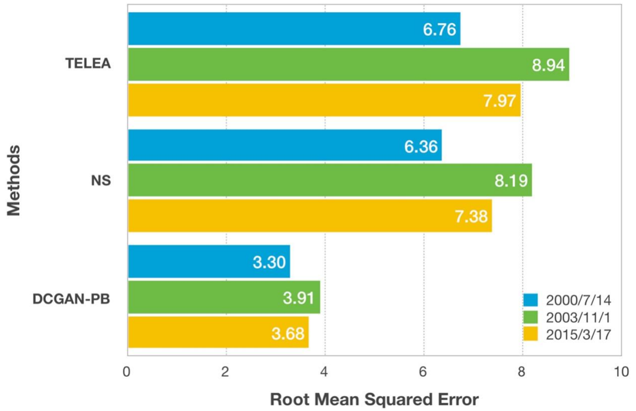
Figure 3.7 RMSE of the recovered TEC values compared with the original IGS TEC maps from three different TEC map completion methods (TELEA, NS, and DCGAN-PB) for three high solar activity cases [Pan et al., 2020].
